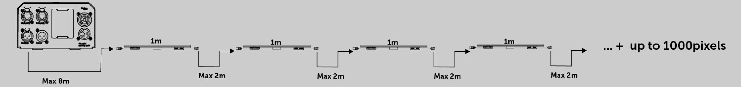
For all other cases, when targeting 1000 pixels on the output for stable operation, maximum system length – cables and units – is expandable with the use of an additional 'CRE:ON HD' unit (switched to 'Bypass' mode) or a 'LEDBLADE Power Supply Unit' (LB-oPSU).
